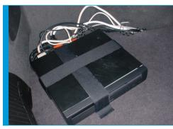
You don't want your equipment to move around while you're driving. The easiest way to prevent this is to use Velcro, which sticks to the carpet or another strip of Velcro. The cables are then tied and secured underneath the carpet for neatness.
