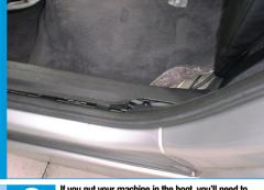
If you put your machine in the boot, you'll need to supply power, audio, video and USB feeds to the rear of the car. Ensure you separate the power cables from the audio feeds to prevent interference. You may want to use a mains three-pin socket and plugs so the system can be quickly removed.
