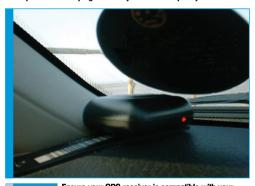
Ensure your GPS receiver is compatible with your intended application. eBay is a good source of USB GPS units, which, when used with a USB hub in the dash, make things easier in terms of cabling. If your car has heatreflective film in the windows, this can affect the quality of the signal.
