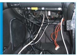
Now to install the system in the car. You'll doubtless have excess cables to stow, along with items such as USB hubs. Space behind the dashboard can be useful here, but be aware of heating or AC elements and don't put anything in there that may be a potential fire risk.
