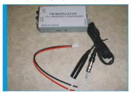
If you have a high-specification car radio, it might have an auxiliary port (possibly left and right phono plug leads), which is the best way to get sound in to your system. Failing this, buy an FM Modulator from eBay for £25-35 – it's easy to connect and all you need to do is tune in your radio.
