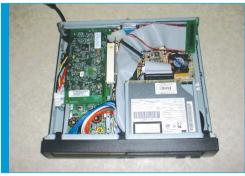
You don't have to think small, as all installations are different, but it helps. We're using a Cubid 2688R case with a VIA mini-ITX board. This case doesn't leave much room inside, but by using smaller components, such as a laptop hard drive, you can pack quite a bit more in.
