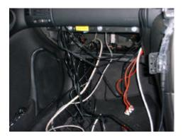
**6)** You more than likely need to supply power, audio, video and USB feeds to the rear of your car if you use this configuration. Make sure that the high voltage cables you will need are separated from the audio feeds to prevent interference. You may want to use a mains three pin socket and plugs to allow the CPU to be quickly removed.
